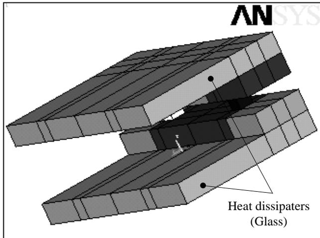
Figure 4. Thermoelectric chain model between two glasses
