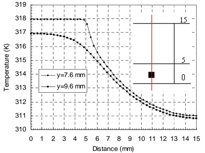
Figure 9. Temperature distribution in the model at the hot dissipater.  $I=4 \text{ A}$ , summer conditions
