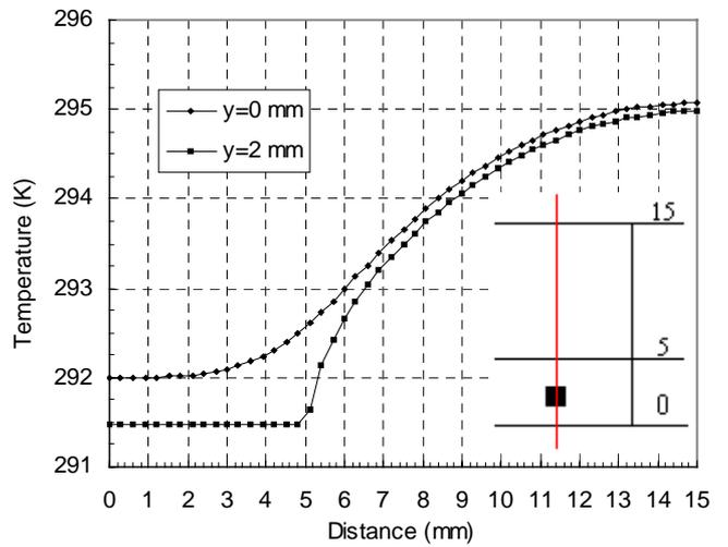
Figure 10. Temperature distribution in the model at the cold dissipater.  $I=4 \text{ A}$ , summer conditions
