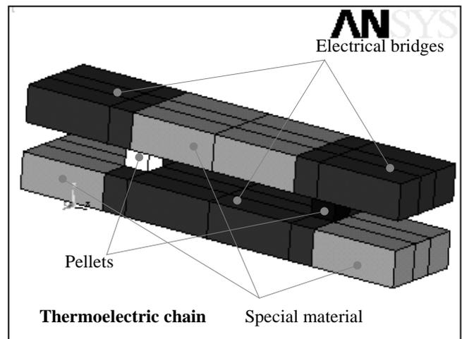
Figure 3. Scheme of one element of the thermoelectric chain
