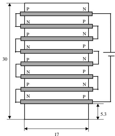
Figure 13. Dimensions of the active thermal wall prototype
