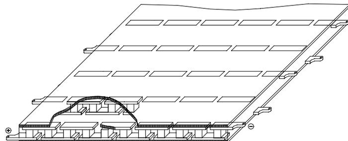
Figure 2. Scheme of the active thermal wall
