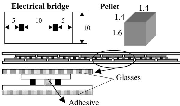
Figure 12. Components of the prototype of active thermal wall, dimensions in mm
