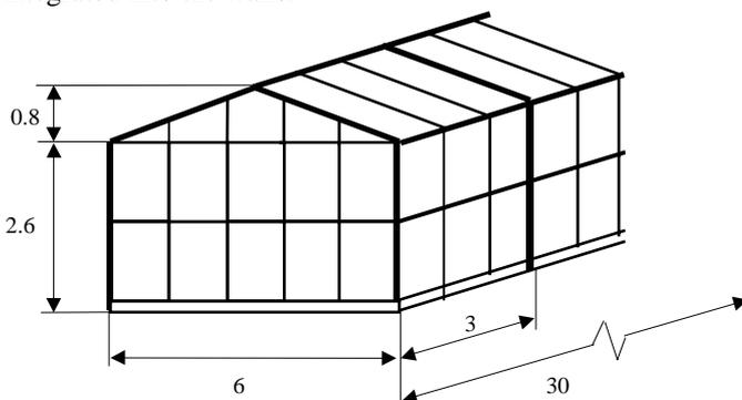
Figure 19. Scheme of the greenhouse, dimensions in m
