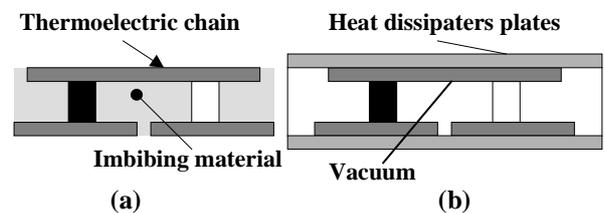
Figure 1. Cross section of a thermoelectric chain
