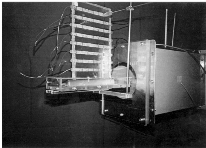
Figure 14. Test bench of the prototype of active thermal wall-1
