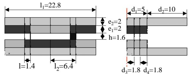
Figure 7. Main dimensions of the model (mm)
