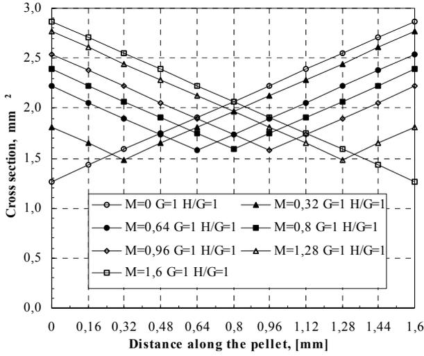
**Figure 5.** Cross section of the pellet when  $G=H=1$  for different positions of the contraction, linear variation.
