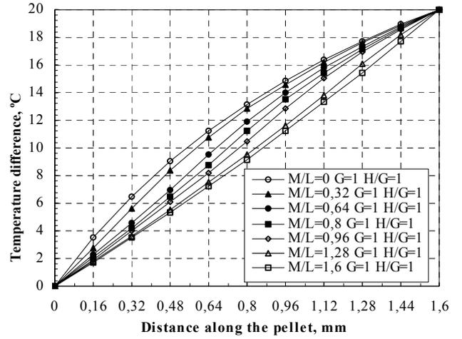
**Figure 8.** Temperature difference ( $T_h - T_c$ ), linear variation,  $T_c = 273$  K,  $G=H=1$ ,  $I_{\phi}|_{max}$
