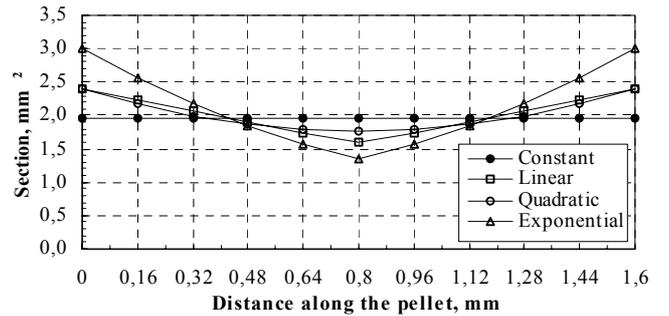
**Figure 11.** Variation of the volume of the pellet with M for different geometries
