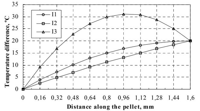
**Figure 4.** Temperature difference along the pellet ( $T_h-T_c$ ) for different electrical currents,  $T_c=273 \text{ K}$ , constant cross section.
