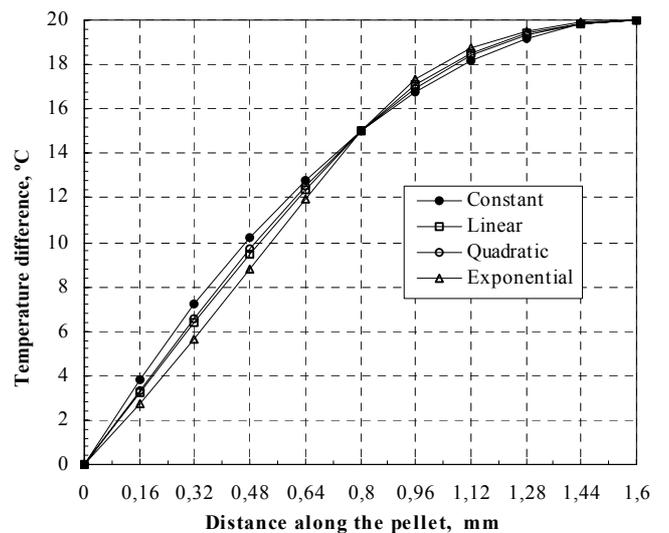
**Figure 12.** Temperature difference, (T<sub>h</sub>-T<sub>c</sub>), T<sub>c</sub>= 273 K,
