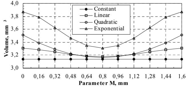
**Figure 10.** Variation of the cross-section for different geometries.
