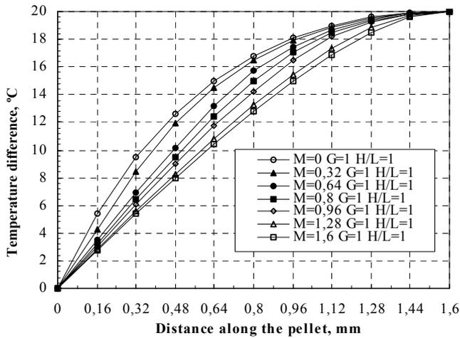
**Figure 7.** Temperature difference ( $T_h - T_c$ ), linear variation,  $T_c = 273$  K,  $G=H=1$ ,  $I_{\phi_c}|_{max}$
