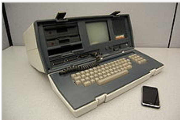
An Osborne Executive portable computer, from 1982, and an iPhone, released 2007. The Executive weighs 100 times as much, has nearly 500 times the volume, cost 10 times as much, and has a 100th the clock frequency of the iPhone.
