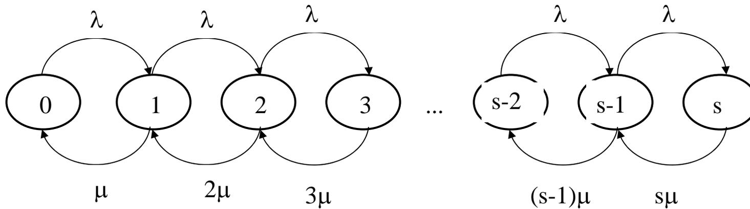
$$C_n = \begin{cases} \frac{1}{n!} \left( \frac{\lambda}{\mu} \right)^n & n \leq s \\ \frac{1}{s!} \left( \frac{\lambda}{\mu} \right)^s \left( \frac{\lambda}{s\mu} \right)^{n-s} & n > s \end{cases}$$
