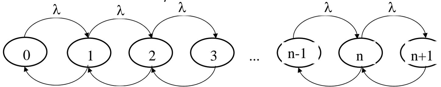
$$C_n = \left(\frac{\lambda}{\mu}\right)^n = \rho^n \quad P_n = \rho^n P_0 \quad P_0 = \frac{1}{\sum_{n=0}^{\infty} \rho^n} = 1 - \rho \quad P_n = (1 - \rho)\rho^n \quad n = 0, 1, 2, \dots^5$$
