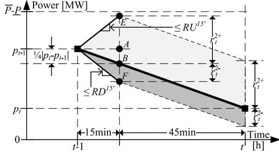
Fig. 3: Relation between secondary reserves, power trajectory and ramps
